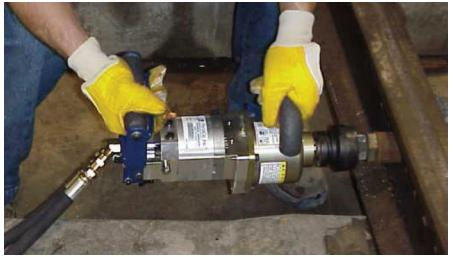
The I" Hydraulic Impact Wrench is designed to tighten and loosen track bolts and lag screws.
